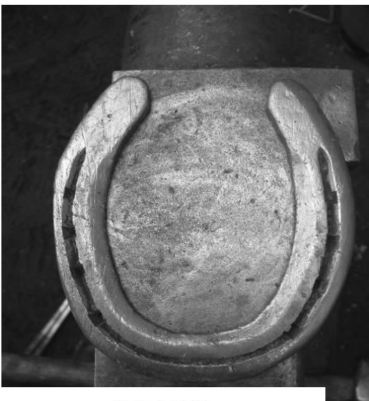
Fig. 54 Observation of horseshoe wear on the lower side
