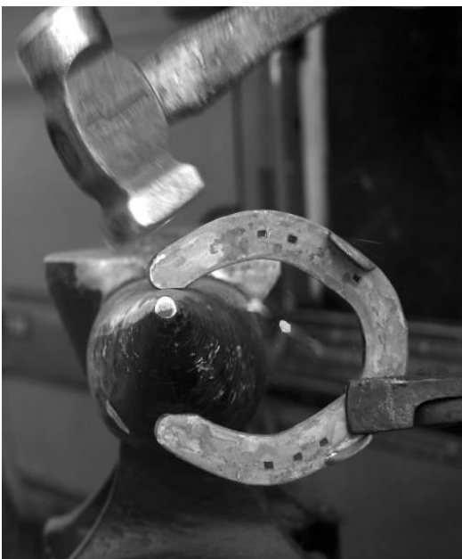
Fig. 61 Turning the horseshoe
