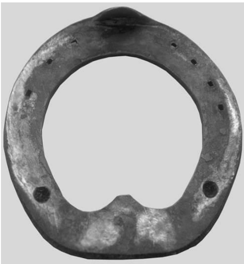
Fig. 63 Straight bar shoe with stud sockets (note the wear on the upper side caused by the movements of the wall and the frog)
